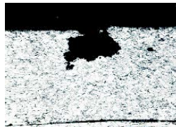
Fig. 2 Detail on the formation of passive film damage (Source Lamiera, April 2008)
